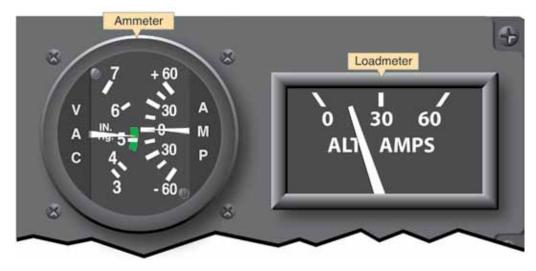
Figure 11-4. Ammeter (left) and Loadmeter (right).
