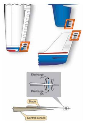
**Figure 11-2.** One example of a static wick installed on aircraft control surface to bleed off static charges built up during flight. This will prevent static buildup and St. Elmo's fire by allowing the static electricity to dissipate harmlessly.
