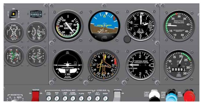
Figure 11-8. Vacuum Failure.
