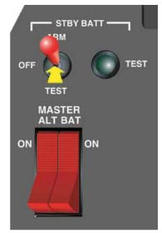
**Figure 11-6.** *Note the double rocker switch and the standby battery switch in this aircraft. The standby battery must be armed to work correctly; arming should be done prior to departure.*
