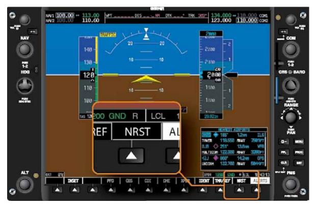
Figure 11-9. The default soft key menu that is displayed on the PFD contains a "NRST" (Nearest Airport) soft key. Pressing this soft key opens a text box which displays the nearest 25 airports.
